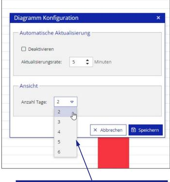
Configuration of the dashboard view is possible for 2 - 6 days, and there is an update every 5 - 60 mins. In the current VTP, only intraday and dayahead are possible here
